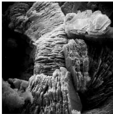
Fig. 3. Layers of naturally occurring phyllosilicate clay as seen under SEM.
